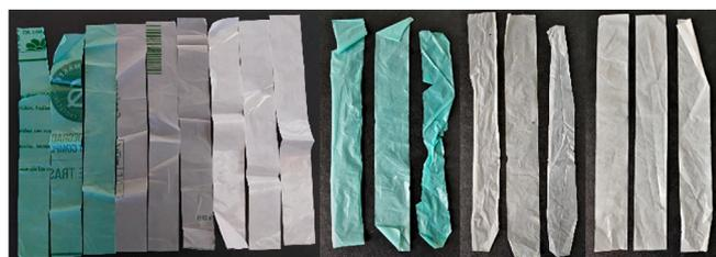
**Fig. 3.** Specimens of biodegradable (BIO1, green; BIO2, beige) and PE bags at day 0 (left) and after 120 days of degradation (right). For each bag from left to right: BEN, PEL, LIT. (For interpretation of the references to colour in this figure legend, the reader is referred to the web version of this article.)
